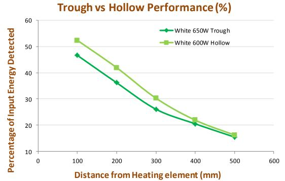
Figure 2: Infrared energy as a percentage of input power for Ceramicx FTE 650W vs. FFEH 600W
